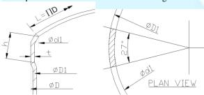
Cross section of steel cover which is going to whirling on angular chamfer
